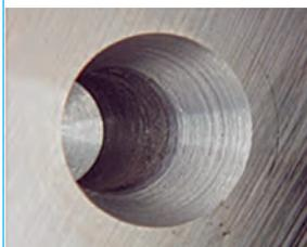
Under the cutting condition stated above, the surface finish of center-drilled hole has been greatly improved. Circularity of center drilled hole as well as run-out tolerance of turning axis has been improved.
