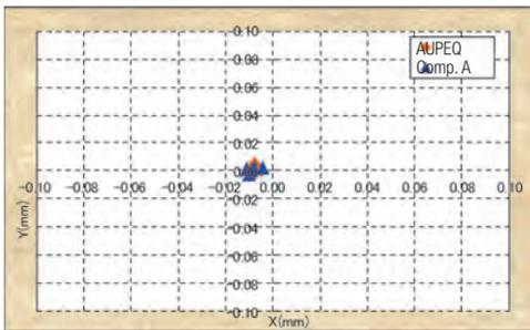
Positioning accuracy on 15° slant surface
