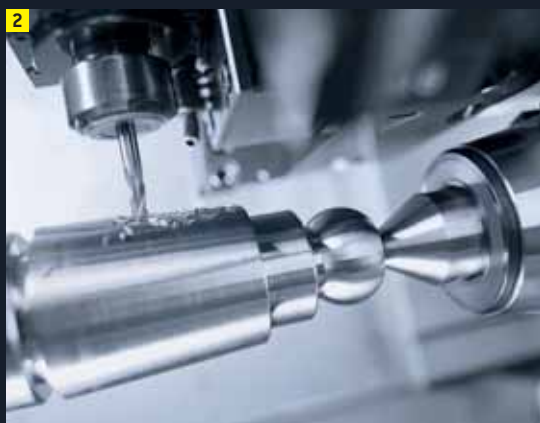
2 Machining with driven tools
