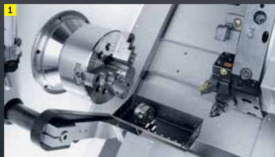
1 Work piece collection device (part of the bar package)
